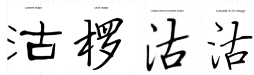
Figure 10. The target character includes the three-dot “water” radical, but the model initially generates the two-dot “ice” radical. The RAG module successfully retrieves the correct three-dot radical and enables the model to produce the desired glyph.
